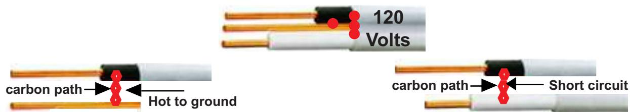
In **120 VAC circuits**, it is not difficult to cause sustained arcing **if there is a carbonized conductive path**.
