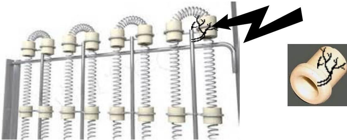
What still appeared was a "worm" on one insulator on the frame to the heating coils. Now my mind started to spin back to the 1950s when I was taught what a "worm" was electrically. An insulator must be maintained and kept clean and dry, if not the dust, dirt or moisture over a period of time will start a tracking path for electricity to follow.
