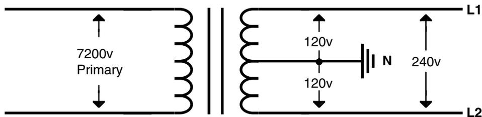
To properly understand and install grounding, the electrician needs to understand AC reactance and how it applies.
