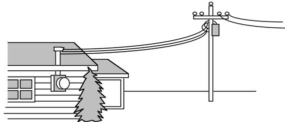
To guard against this hazard, the system is required to be effectively grounded. By connecting the neutral conductor to earth, no conductor of the grounded secondary circuit could have a potential greater than the normal circuit voltage.
