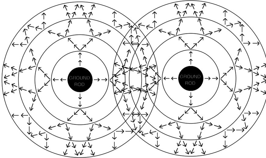
If you had two ground rods connected in parallel spaced 10 feet apart, the resistance is lowered approximately 40%. If the spacing is increased to 20 feet apart, the resistance is lowered to approximately 50%.
