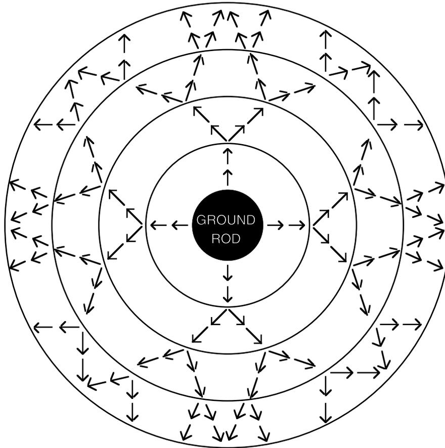
The earth shell nearest to the ground rod has the smallest surface area and offers the **greatest** resistance. The next earth shell is a little larger in area and offers **less** resistance. And each shell on out offers less resistance and so on. Eventually, a distance will be reached where additional earth shells hardly add any resistance to the earth surrounding the ground rod.
