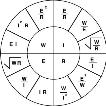
The Ohm's law circle actually applies to DC (direct current) pure resistance. AC (alternating current) has two components not found in a DC circuit that add opposition to the normal flow. These two components are called "inductive reactance" and "capacitive reactance."
