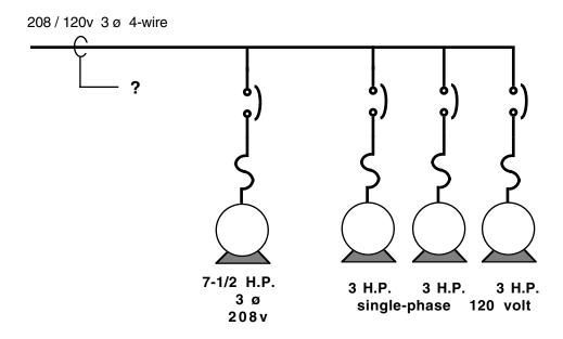
Solution: Table 430.250: 7 1/2 hp, 208v F.L.C. = 24.2 amps. Table 430.248: 3 hp, 120v F.L.C. = 34 amps. The largest motor is the 3 hp at 34 amps. 34 amps x 125% = 42.5 amps + 24.2 amps = 66.7 required ampacity. Table 310.16 would require a #4 TW copper conductor minimum.
