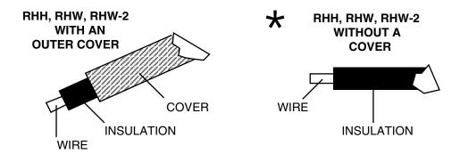
Example: What is the area square inch for a #12 RHW conductor without an outer covering?
