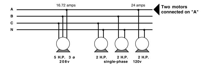
When the exam question mentions a three-phase motor with **single-phase 120 volt motors**, draw a sketch and make the motor connections for the proper voltages (208v is line to line and 120v is line to neutral). Now count how many motors you have on the **SAME** conductor. This is the **key** in answering this type of question. The error generally made is counting four motors instead of **two**.
