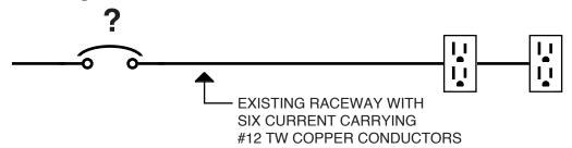
Branch circuits rated 10 amperes shall not supply receptacle outlets.
