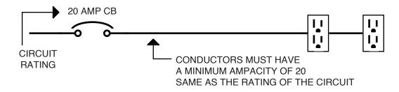
A #14 TW conductor has an **ampacity** of 15, and the \* asterisk, which refers you to the bottom of Table 310.16 states a #14 conductor can only be fused at a maximum of 15 amps (240.4D). A #12 TW with an ampacity of 20 would be protected at 20 amps and would be the correct selection of conductor for this receptacle circuit.
