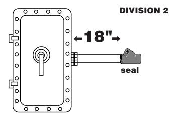
**501.15(B)(2).** Class I, Division 2 boundary, the seal is permitted on either the Division 2 or nonhazardous side of the boundary. It must be installed in a manner that will minimize the gas or vapor that can enter the conduit system within the Division 2 location and be communicated beyond the seal.
