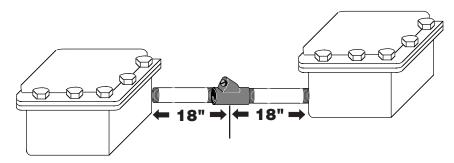
*Note:* According to UL Hazardous Location Equipment Directory, no splices are permitted within a seal.
