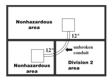
**501.15**(B)(2) Exception 2. No seal is needed in the conduit run from a Division 2 to a nonhazardous area where a transition is made in the nonhazardous location from a conduit to cable tray, cablebus, ventilated busway, Type MI cable or open wiring.
